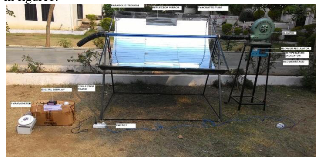
Figure 1. Experimental set up of parabolic trough collector
